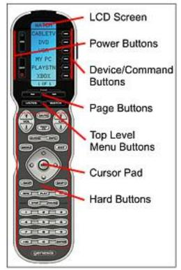
The Light Button on the right side of the remote illuminates the LCD screen and hard buttons.
